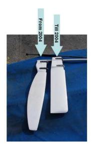
The following figure shows the evolution of centerboards at Duvoisin and the design of the centerboard that is in the boat
